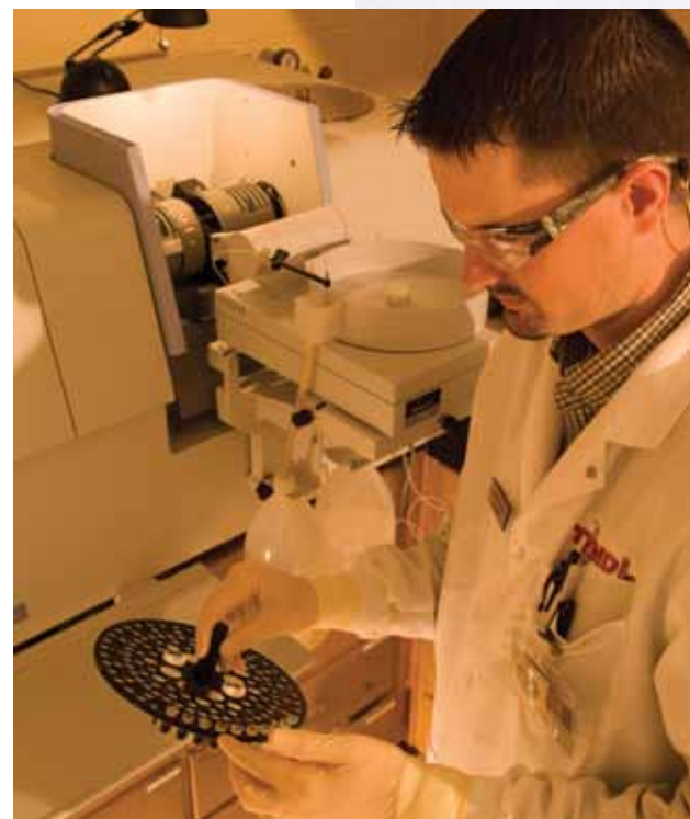
ABOVE: Travis Mays, TVMDL veterinary toxicologist, loads samples into a graphite furnace atomic absorption spectrophotometer, which measures lead, arsenic, and selenium in blood, serum, or liver samples.
