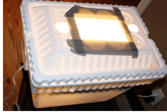
Figure 4: Cooler lid with glass viewing window and two cork-sized holes for ventilation.
