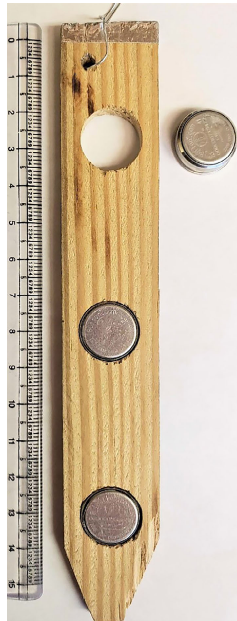
FIGURE 1 A complete iButton stake that will measure soil depths 5, 10, and 15 cm when installed with the top of the stake (picture left) 2 cm below the soil surface
