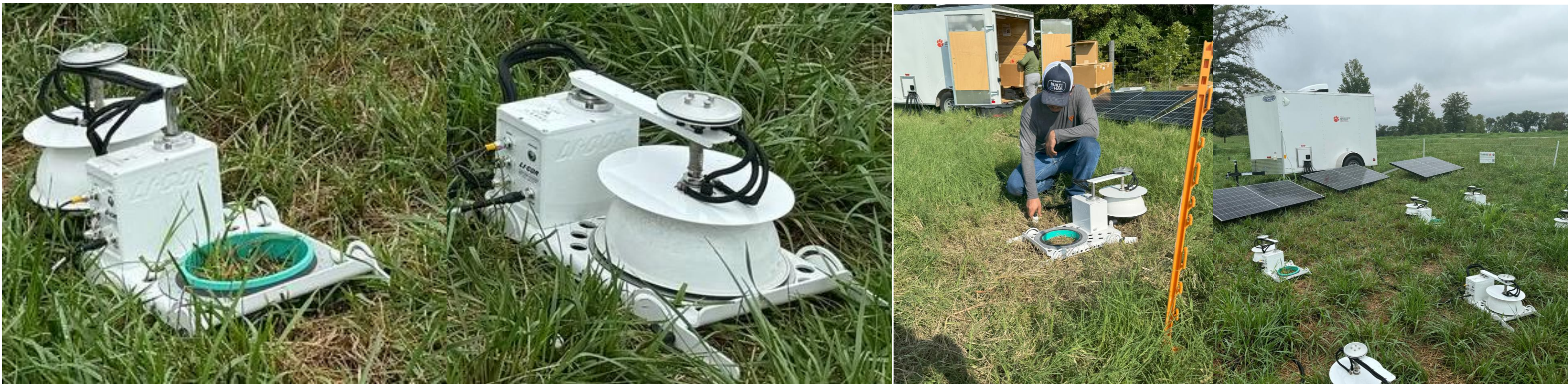
Figure 2. Chamber installation (left), soil temperature sensor installation (middle), and setup of deployment on-farm (right).
