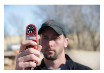
It is extremely important to know what the onsite weather conditions are prior to conducting the burn. This can be accomplished with a digital hand-held weather device. (Photo courtesy T. Johnson)
