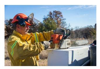
When using a chainsaw, safety should be your top priority. Chainsaw operators should wear full protective gear. Care should be taken when operating the chainsaw near hot spots on the tree due to the air movement created by the saw, which can cause flames to flare-up injuring the operator or damaging the saw. (Photo courtesy J. Weir)
