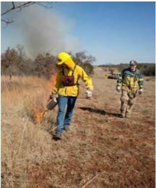
The most widely used ignition device is a drip torch. Drip torches use a mixture of diesel and gasoline. A mixture of 50:50 diesel to gasoline works very well for temperatures ranging from 35 F to 75 F. When temperatures are higher than this, a mixture of 60:40 or 70:30 diesel to gasoline is recommended to reduce the volatility of the gasoline and to help the torch operate properly. (Photo top two photos courtesy J. Weir, middle photo courtesy J. Bradley, bottom photo courtesy T. Johnson)
