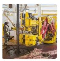
industry, improving efficiency, accuracy, and safety. The Iron Roughneck is a versatile and reliable machine that automates the process of making tubular connections, minimizing hazards, saving time, and
