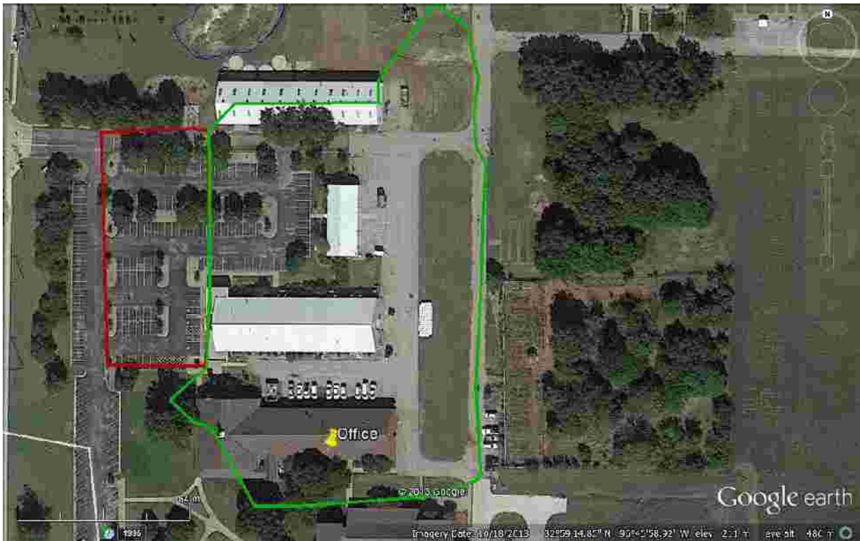
Figure 55. Watershed of the east side of the detention pond (green) and the bioretention area (red line).
