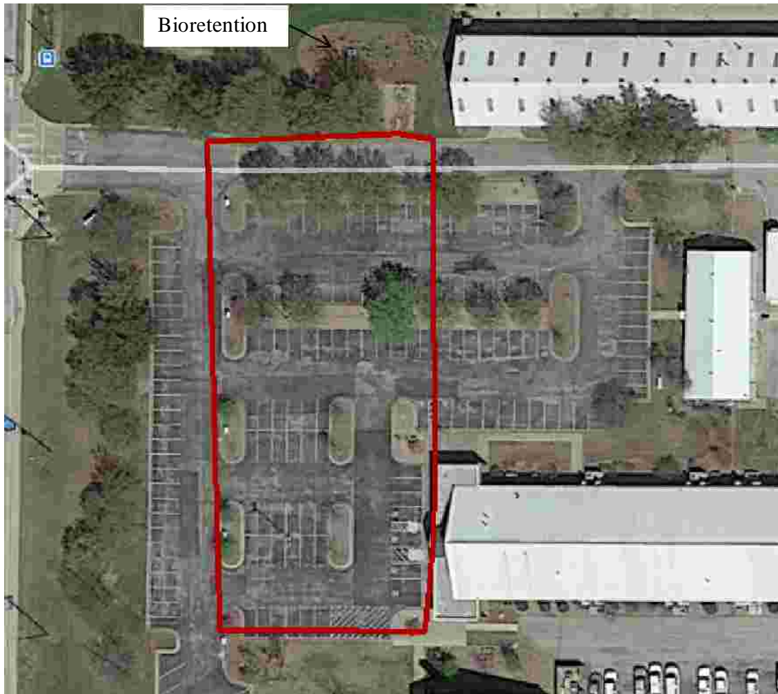
Figure 3. Bioretention area and its watershed (Redline)
