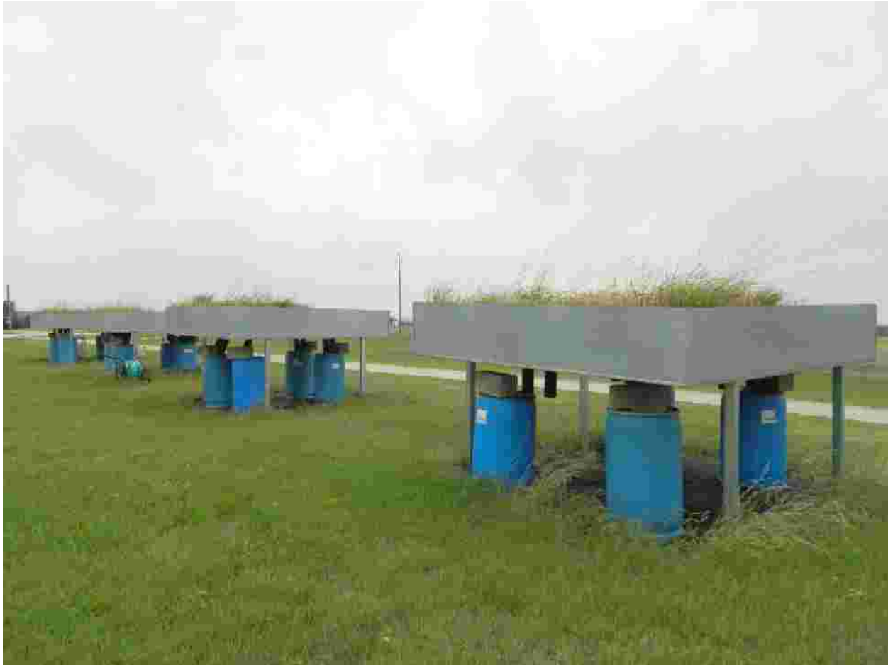
Figure 8. Green roofs and collection system
