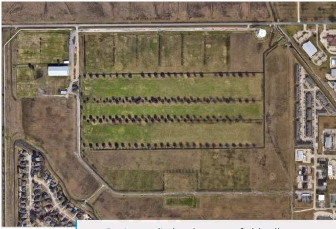
Drainage ditches between fields allow water to flow away from recreation areas efficiently. Imagery ©2024 Google, Airbus, CNES / Airbus, Maxar Technologies, U.S. Geological Survey, USDA/FPAC/GEO, Map Data.
