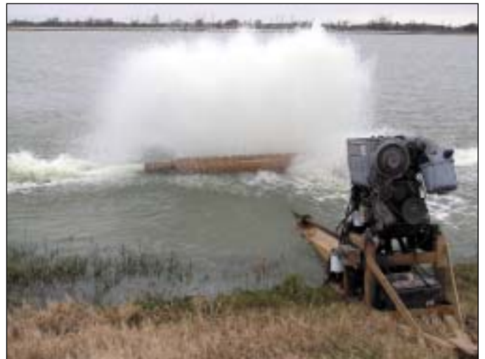
Figure 17. Pump-sprayer or “bankwasher” type diesel aerator.
