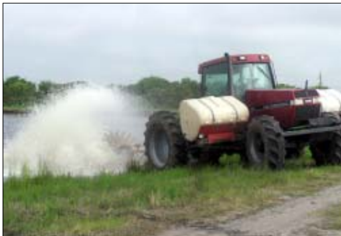
Figure 15. Tractor powered (PTO) “sidewinder” type paddlewheel aerator.
