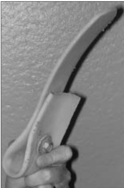
Figure 4. High-density polyethylene plastic hatching paddle.
