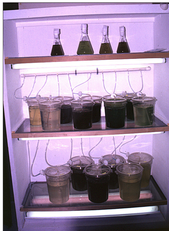
Figure 6. Starter cultures in 500-ml flasks and 2-L and 4-L polycarbonate containers. Note that the flasks are not aerated, but the larger containers are aerated (with CO 2 added) and contain an in-line air filter (J. Scarpa, Harbor Branch Oceanographic Institute).
