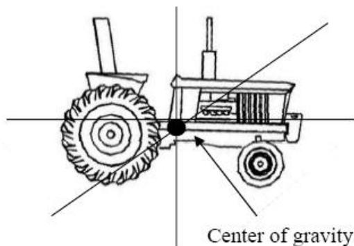
**Center of gravity** is defined as the point of equal weight distribution. This means that 50 percent of the tractor's weight is distributed in front of this point and 50 percent behind. This same principle applies from side to side and top to bottom. On any given tractor, the center of gravity will vary under different conditions.
