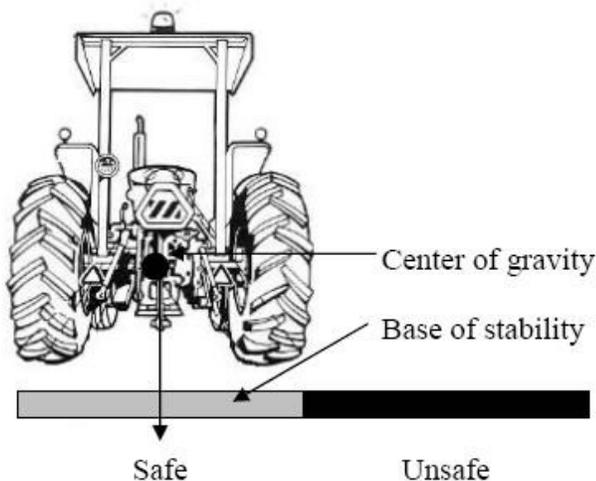
However, circumstances that displace the tractor's center of gravity from within this safe zone will result in either a side or rear rollover incident.
