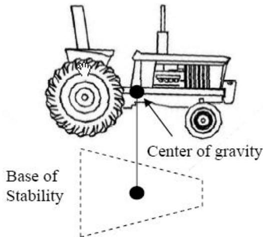
As long as the tractor is operated in a manner whereby the tractor's center of gravity is within the base of stability, the tractor is not subject to rollover.
