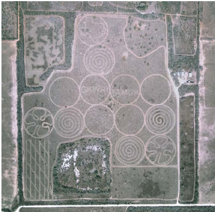
Figure 3. Post-treatment vertical natural color aerial photography (flown March 1, 2006 by Lanmon Aerial Photography, Inc.) showing how well the plan was implemented using GPS and mobile GIS software running on a field computer mounted inside the tractor cab.
