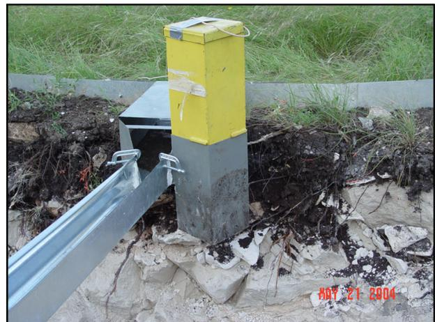
Figure 3. The 15.25 cm (6 in.) H-flume with stilling well used to quantify surface runoff at the inter-canopy plot flume assembly. The gutter extension shown on the flume outlet conveys water over the trench and away from the plot. The grass cover shown in the background is typical of cover throughout the plot.
