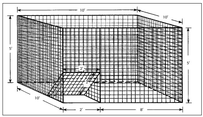
Figure 3. Multi-catch live trap for feral hogs.
