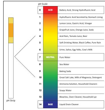
Figure 11. pH strip and pH scale.
