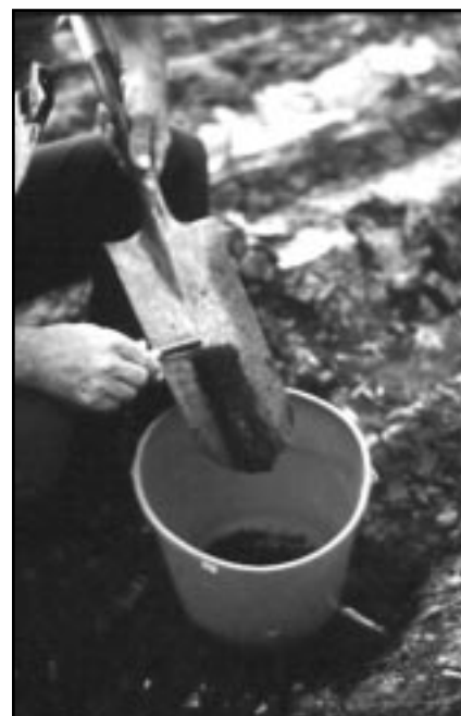
Figure 1. Soil sampling is the most important step in soil testing. Above is an example of a 1 x 1 x 6-inch core taken with a spade.
