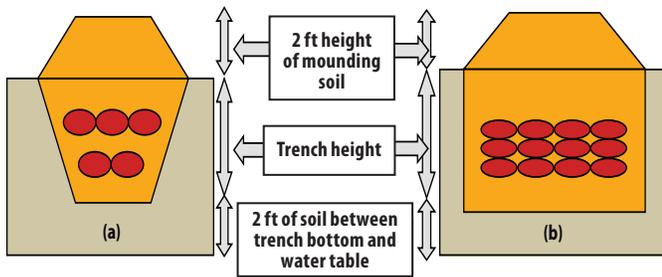
**Figure 4.** Layout of trapezoidal (a) and rectangular trench (b) for burying carcasses.
