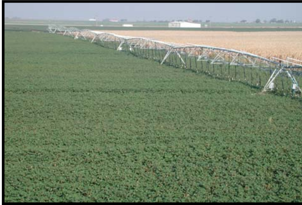
Fig. 1. Variable-rate irrigation system used in cotton and corn site-specific irrigation experiments, Helms Farm, 2004.
