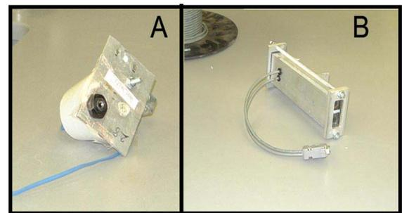
Fig. 1. Cases developed for the TIR sensors (A) and pairs of RED and NIR sensors (B).
