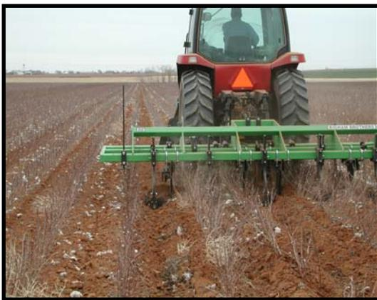
Fig. 1. TerraTill plow used for deep tillage of SDI cotton plots, 2003.
