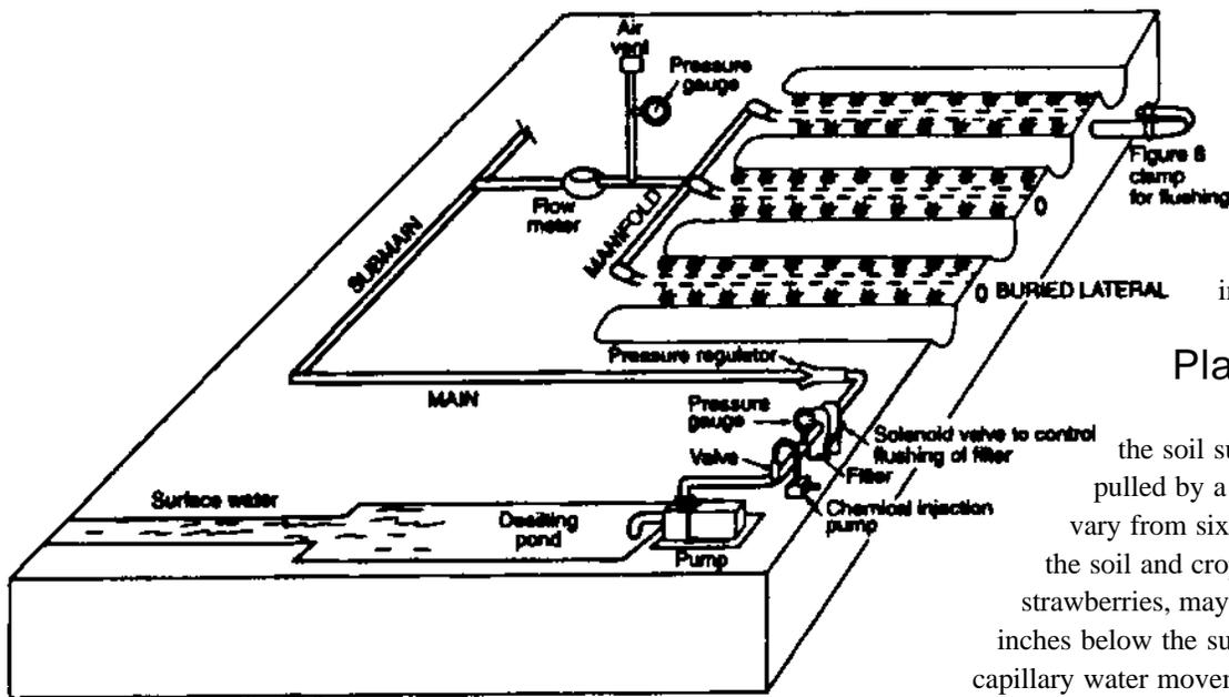
Figure 1: A typical subsurface microirrigation field layout.
