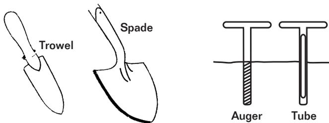
The selected tool must be able to cut a slice or core through the desired layer of soil as illustrated in Figure 4. The objective is to obtain a cross section of the plowlayer or layer being subsampled.
