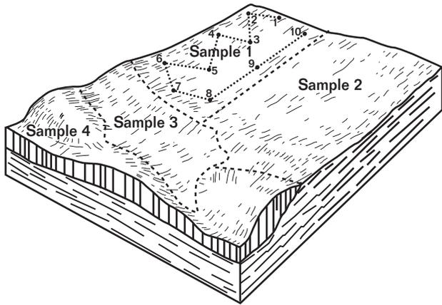
Factors that will affect results include sampling tools, number of subsamples, depth of sampling, and soil compaction and moisture.
