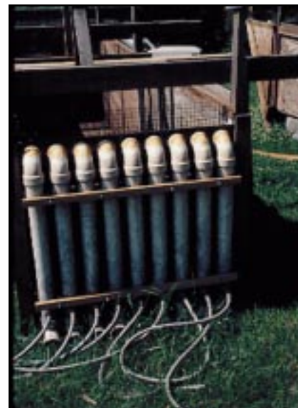
Figure 4a. Air-lifts attached to a sheet of plywood at the front of raceway, showing garden hose attachment at a water depth of 32 inches.
