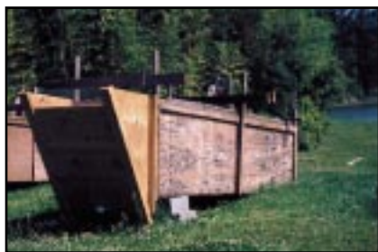
Figure 3a. IPR (out of the water) built from treated plywood showing external frame and attachment of tube settler.
