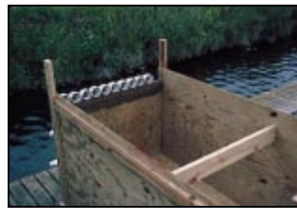
Figure 2. IPR (out of the water) showing position of air-lift system and eddy board.
