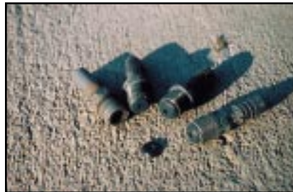
Figure 5a. PVC tubing connectors with restriction orifice(s).
