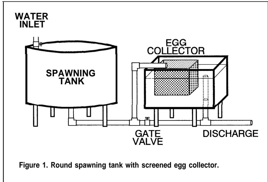
Figure 1. Round spawning tank with screened egg collector.
