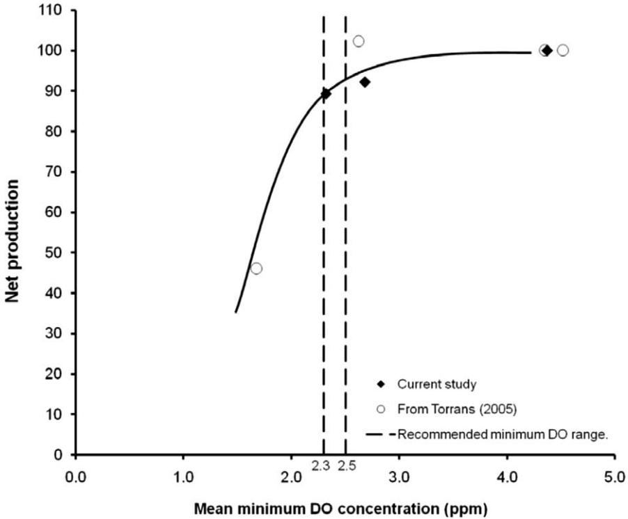
FIGURE 5.—Effect of minimum dissolved oxygen (DO) concentration on the net production of channel catfish. The DO concentration is the treatment average minimum concentration for June–September; net production is expressed as a percentage of that in the high-oxygen (control) treatment. Data derived from Torrans (2005) are presented for comparison. The dashed vertical lines show the range of recommended minimum DO concentrations.
