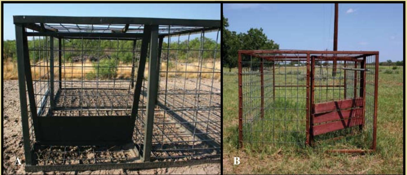
Figure 3. Common box trap designs featuring a lifting (top-hinged) gate (A) and a swing (side-hinged) gate (B).
