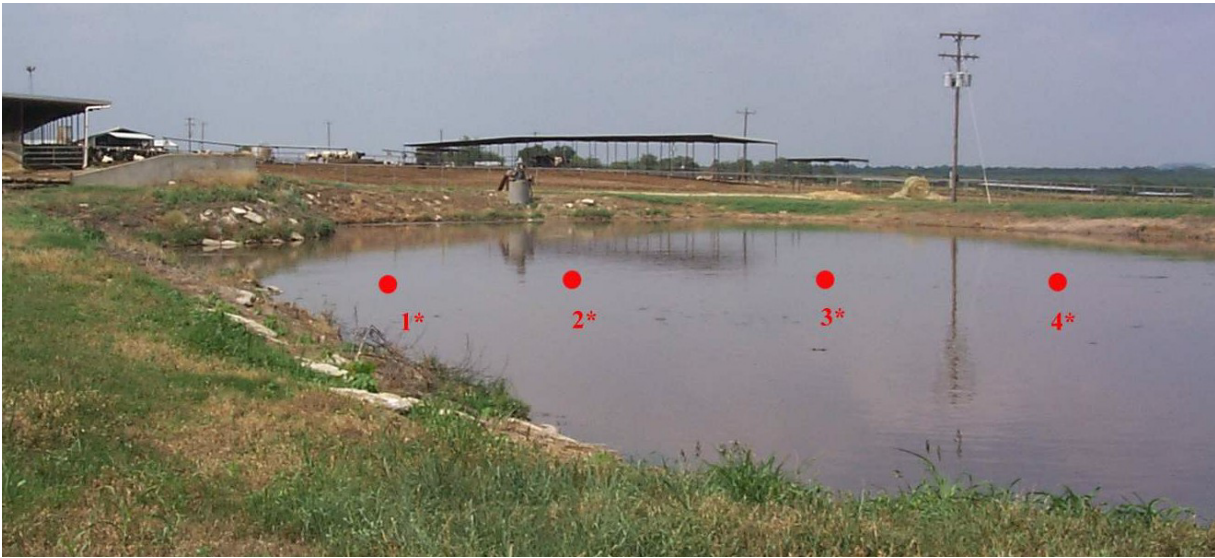
Figure 2. Sampling scheme of a representative lagoon with sludge depths and chemical analysis performed at each location indicated (fifth sampling location not shown).
