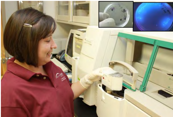
RiboPrint genetic fingerprinting of E. coli bacteria at Texas AgriLife Research Center, El Paso, Texas. Insets, E. coli isolated from water and fecal samples
