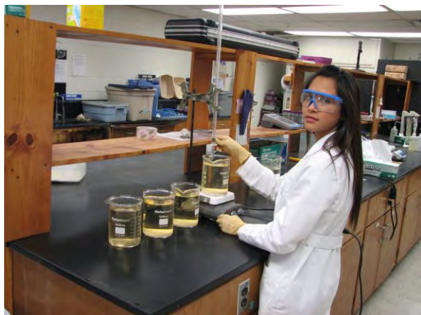
Ammonium being removed (precipitate at the bottom of the beaker) from BPF
