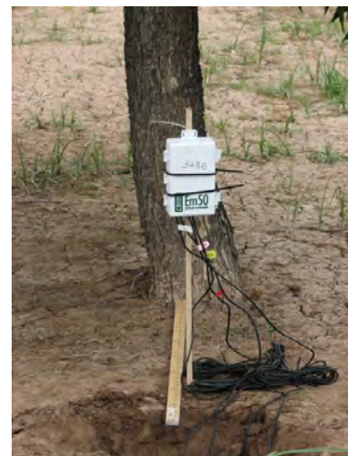
Example of a soil moisture sensor installed in the field
