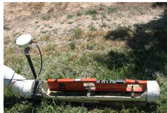
Electromagnetic induction meter fitted with GPS unit
