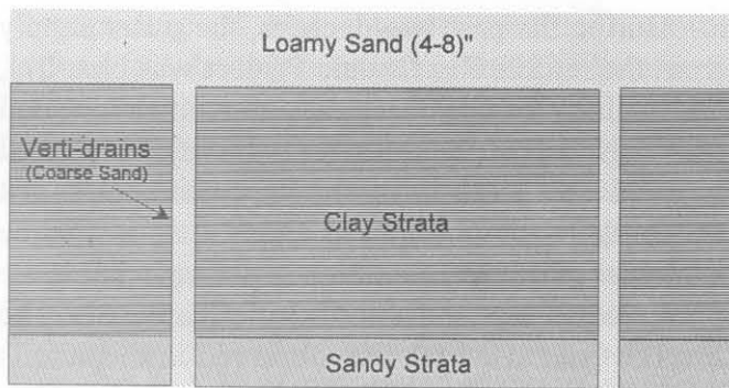
Fig III-5. A cross-sectional view of ground preparation used on clayey soils with sandy sub-strata below.
