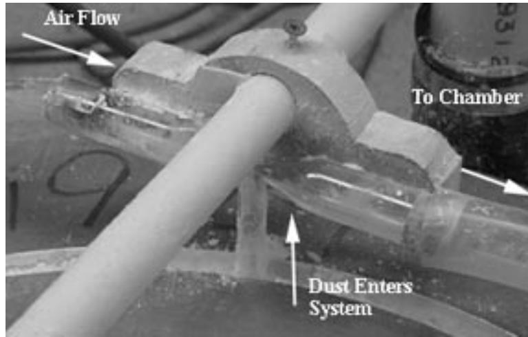
Figure 4. Venturi tube that is used to move dust from disk into chamber.
