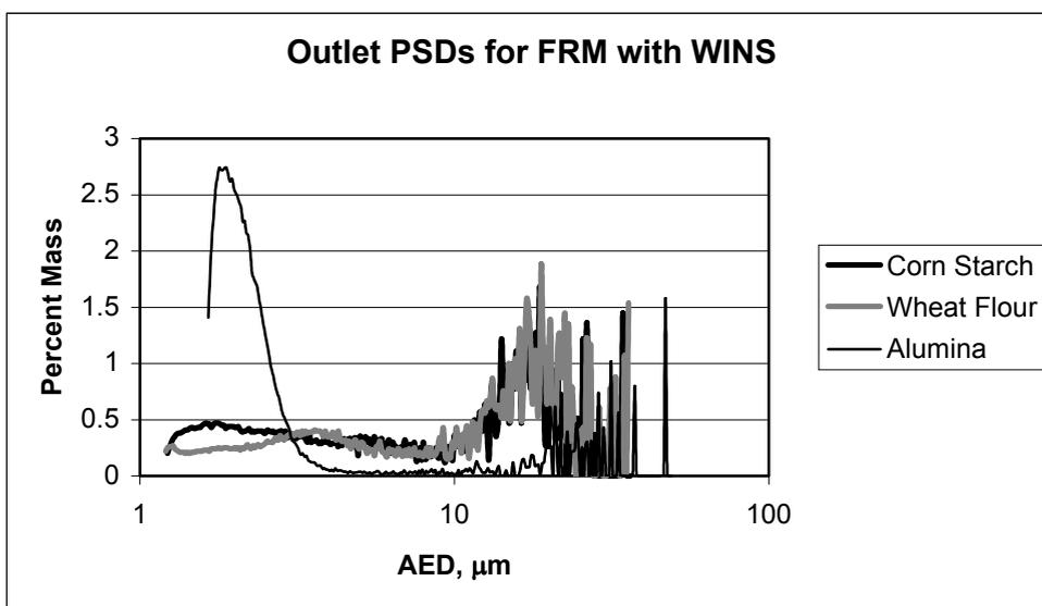
Figure 13. FRM with WINS outlet PSDs for each of the three dusts used in testing.
