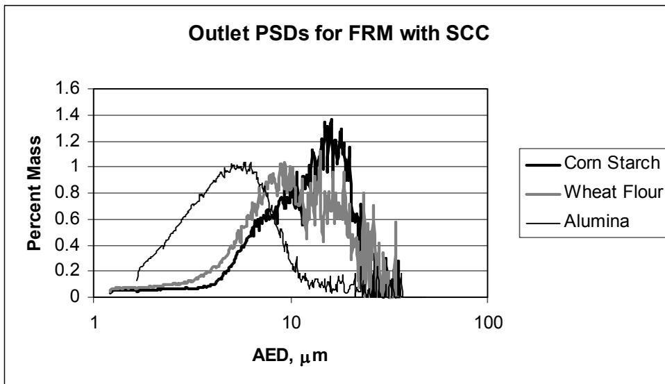
Figure 12. FRM with SCC outlet PSDs for each of the three dusts used in testing.
