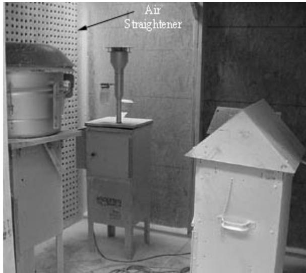
Figure 3. Inside view of chamber, showing sampler set-up and air straightener located between one transition and cube body of chamber.
