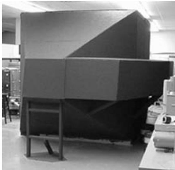
Figure 2. Back view of dust chamber showing one 45° transition and the connected duct.
