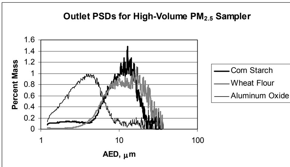
Figure 11. High-Volume PM<sub>2.5</sub> sampler outlet PSDs for each of the three dusts used in testing.
