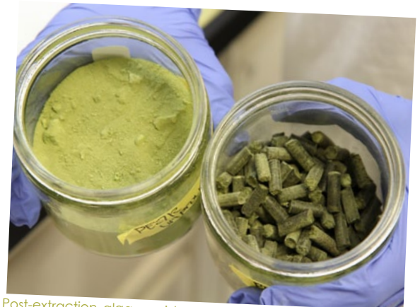
Post-extraction algae residue powder is processed into small pellets and fed to cattle.
