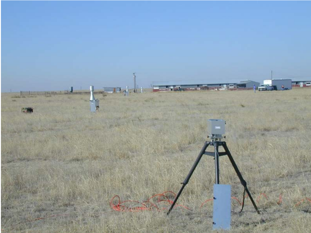
Figure 1. Calibrating the open-path transmissometer at Nance Ranch, Randall County, TX. Transmitter unit is on the tripod in the foreground; also note three pairs of federal reference method PM monitors ( PM_{10} and TSP) along the open path. Receiver unit is barely visible on a white pedestal between the most distant PM_{10} monitor and the end of the maroon-and-white barn. Calibration path length was 300 m.
