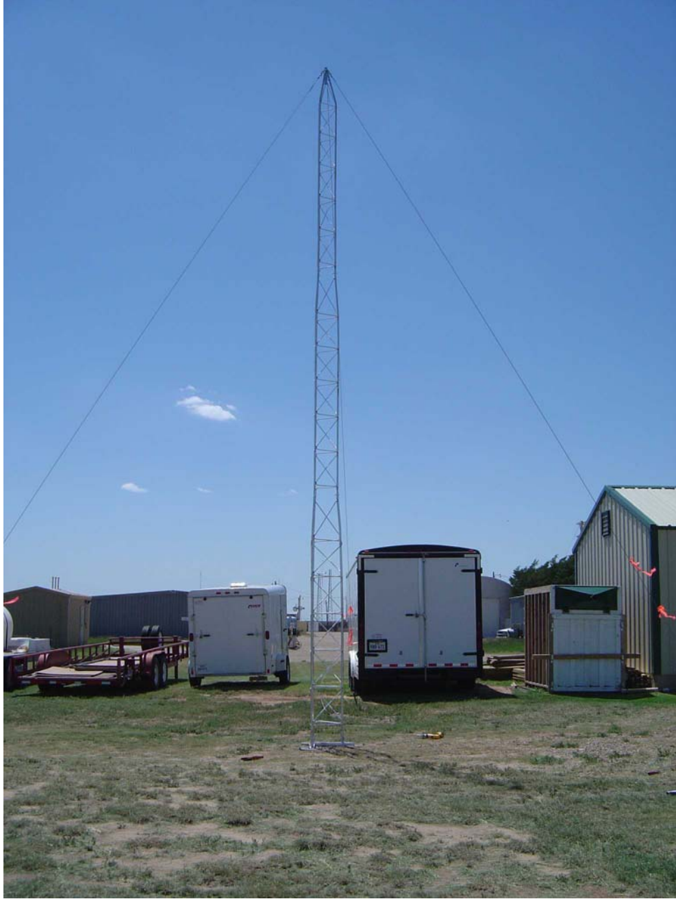
Figure 5. Ten-meter tower to be used to elevate transmitter for long-path (>1 km) transmissometer deployment.
