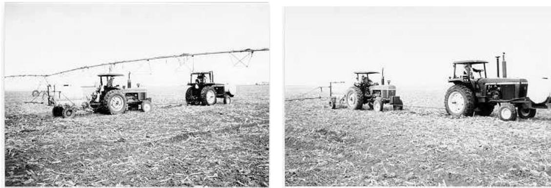
Figure 5. Two perspectives on the tandem-tractor arrangement used to ensure precise application of liquid inorganic fertilizers through a spray rig. The rear tractor maintained pump pressure and PTO speed; the front tractor was responsible for maintaining the proper ground speeds for different application rates.
