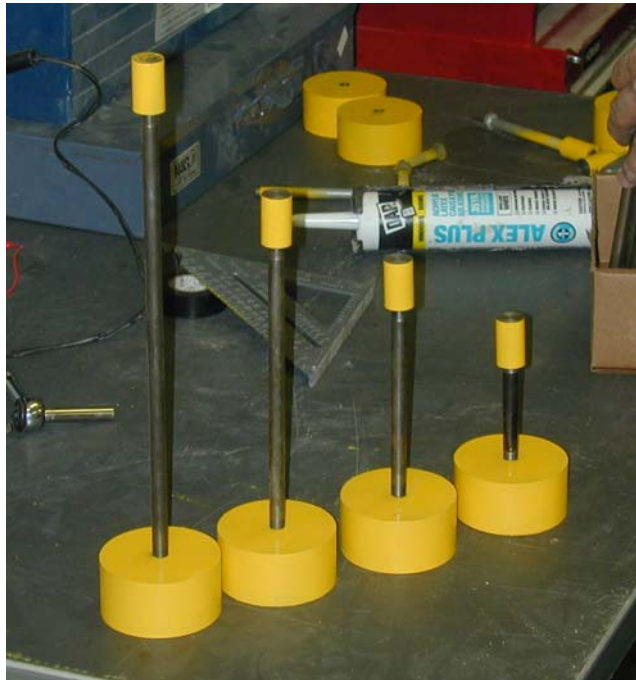
Figure 2. Standardized steel weights in a variety of shaft lengths used to vary the height from which the weights are dropped. The yellow segment at the top attaches directly to the contact face of the electromagnets.
