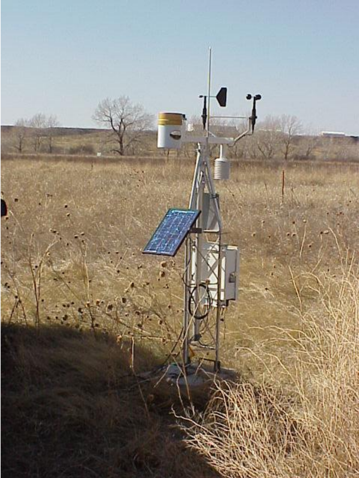
Fig. 4. Weather station located at the ARA release site at Fort Carson, Colorado. Another weather station is located at the Duck Pond release site. These stations collect continual climatic data. The data is downloaded onto a portable computer at regular intervals and kept for future reference and analysis.
